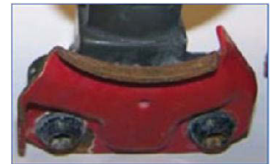
Powder Coated Steel Connector Plate
