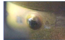
Connector Dimple with Wear
