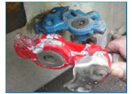
Powder Coated – Corrosion has begun where the coating has chipped
