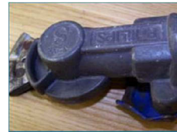
Anodized – Virtually no corrosion on the body
