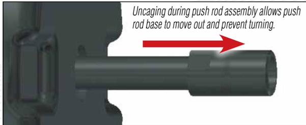
2. Install the TSE-REX™ fixed clevis or threaded push rod kit on the push rod base support collar.
