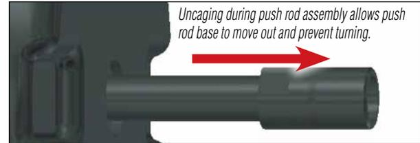
2. With an 11/16" wrench, loosen (counter-clockwise) and remove the support collar from the push rod base. Considerable effort may be necessary to overcome applied threadlocker.
