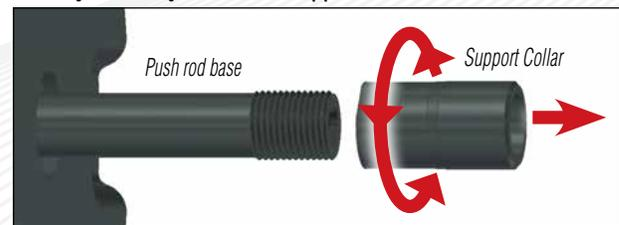
3. Remove excess threadlocker from the threads of the push rod base, if necessary.
