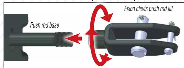
5. With an open end 11/16" wrench, tighten to 1/8 turn past hand-tight.
