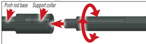
3. If an open end torque wrench (1/2") is available, tighten to 25–30 ft-lbs (34-41 Nm). If using a plain open end 1/2" wrench, tighten to 1/8 turn past hand-tight.
