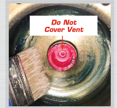
Fig. 3: Paint in the inside of stamped steel hub cap will grease
