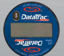
Display turns off when vibration is detected (vehicle moving) to conserve energy.
