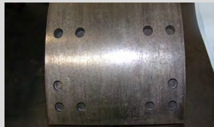
OEM Friction Supplier B; 260 Stops Light heat check; No cracks noted
