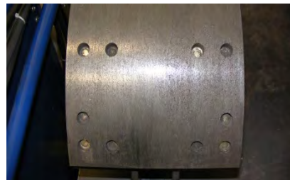
Popular Aftermarket Supplier C; 217 Stops Light heat check; No cracks noted
