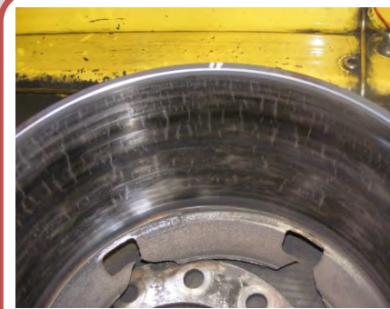
Popular Aftermarket Supplier D; 60 Stops Heavy heat check & hot spotting. Drum catastrophically failed
