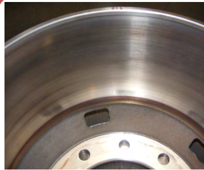
Popular Aftermarket Supplier C; 217 Stops Light heat check; No cracks noted
