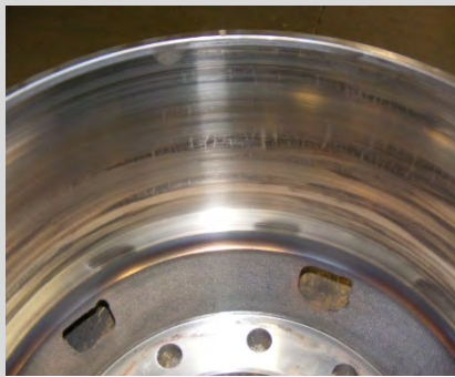
OEM Friction Supplier A; 351 Stops Light heat check; No cracks noted
