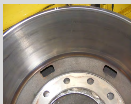
OEM Friction Supplier B; 260 Stops Light heat check; No cracks noted
