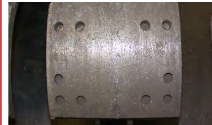
Popular Aftermarket Supplier D; 60 Stops Heavy heat check & hot spotting. Drum catastrophically failed
