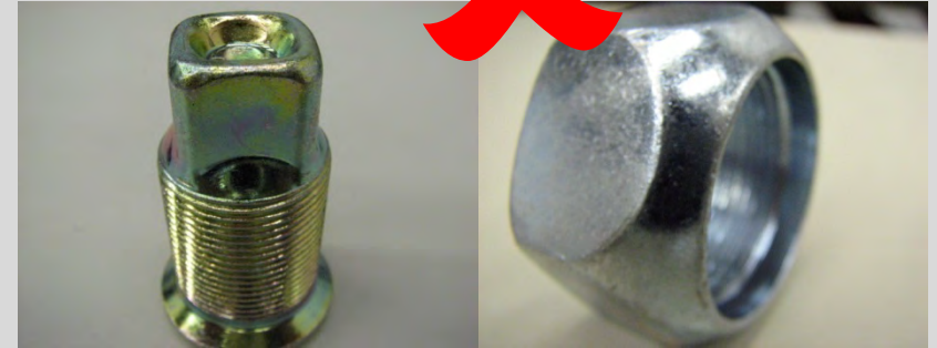
Inner and Outer Cap nuts for Ball-Seat (BSN) Mounting Systems – Do NOT use ball-seat nuts with Hub Piloted Wheels
