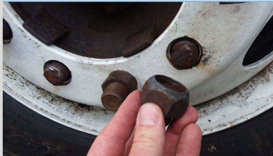
Inner and Outer Cap nuts for Ball-Seat (BSN) Mounting Systems – Do NOT use ball-seat nuts with Hub Piloted Wheels
