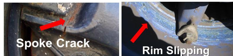
4. Evidence of welding repair in any area—there should be none. The flange of the rim should not be bent or distorted from its original shape or contour.
