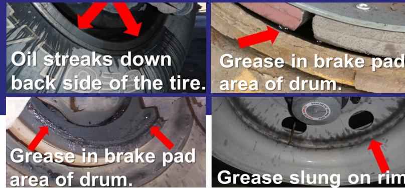
The back side of the wheel can be inspected by looking from the opposite side of the unit.
